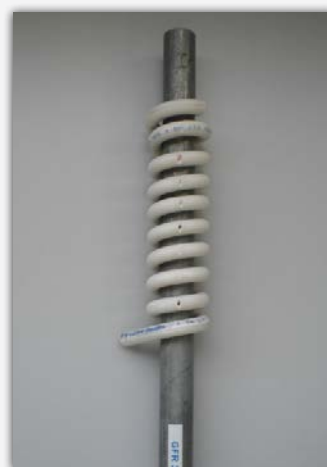
Stress bending test at high temperature with high grade compound
